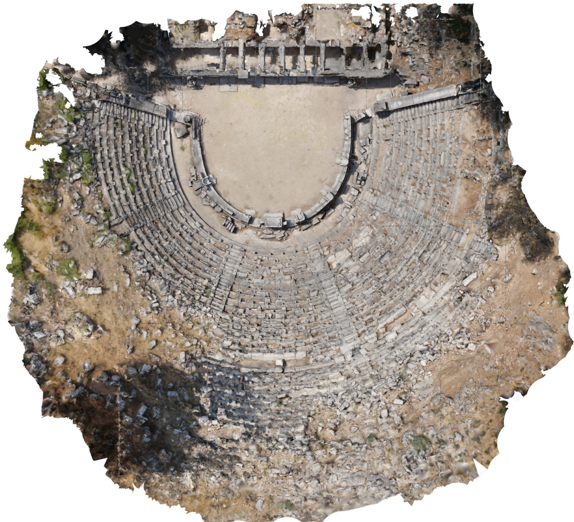
Figure 2. Plan view from the SfM/IM photogrammetry, final restitution of the photogrammetric model of the existing state exported from RealityCapture after the alignment of all components (drone and ground photos) through control points.
